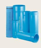
strength - Excellent mechanical properties thus is capable of withstanding the hydraulic pressure, the pipes are subjected to during construction of well • uPVC Casing pipes have trapezoidal threads which provides easy and strong joints • uPVC screen pipes has horizontal slots which enables laminar flow into the well ensuring higher permeability & reducing well entrance.
